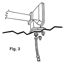
6. Connect the other end of the flexible inlet hose to the valve that will provide air from the tank on-board system
