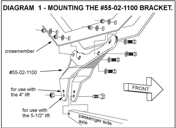
□ Install and torque the factory axle eye pivot bolt (120-150).
