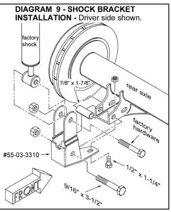
OD x 1-7/8" sleeve inside the existing mount, then install the supplied 9/16" x 3-1/2" bolt through the relocation bracket, existing mount, and sleeve as shown. Snug the bolt with a 9/16" nyloc nut, but do not fully tighten at this time.
