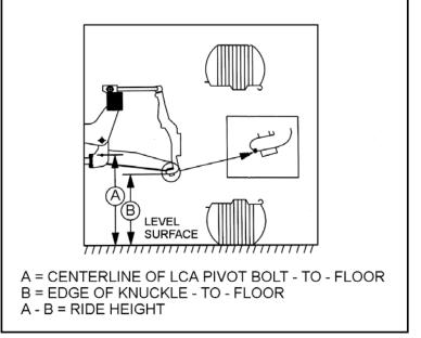
adjusting bolt to resettle the torsion bars. This will ensure accurate adjustments. Adjust height 3/8" to 1/2" above the final desired ride height, since the bars will settle slightly after the vehicle is driven.
