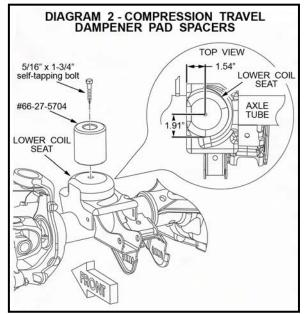
dimensions in Diagram 2; note that the compression pad spacer is installed slightly outboard of seat center. Drill at the marked location using a 17/64" bit.
