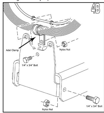
and secure using factory hardware (75).
