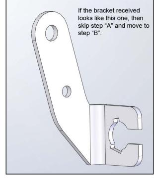
NOTE: If SL brackets 55-13-3480 and 55-14-3480 have a sloted hole for the brake lines to slide in, skip step "A" and move to "B".
