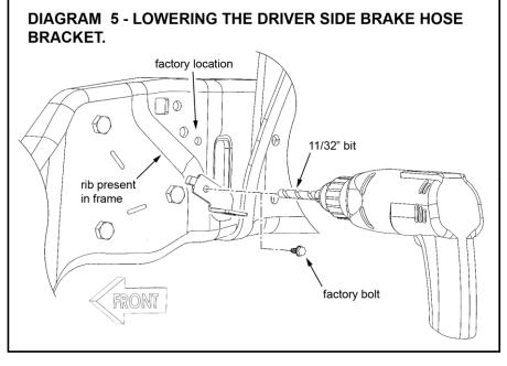
this location. Carefully reform the metal brake line so that the alignment tab in the brake hose bracket engages the existing hole in the frame as shown. Using the bracket as a template, mark the location of the second hole to be drilled.
