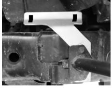
Fig. 3: Reservoir bracket passenger side
