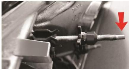
Next locate the tools that will be needed to adjust your headlamps. **Note: Please do not ever use power tools on your adjusters this may cause severe damage to the internals of your lights.**
