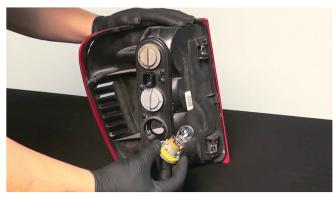
5) Remove reverse lamp bulb from the OEM tail light. Never touch exposed bulbs with bare hands.
