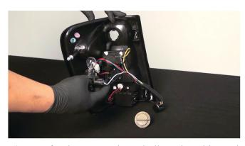
6) Transfer the reverse lamp bulb to the white and black wire reverse lamp socket of the Spyder tail light. Reinstall the socket, then your Spyder tail light is ready to install.
