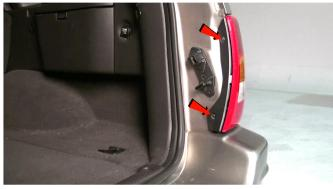
2) Open the tail light access panel by releasing the two tabs.
