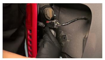
4) Disconnect the tail light wiring harness. Push up on the red tab to unlock the harness, disconnect the harness and remove the OEM tail light.
