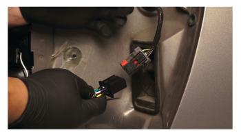
7) Connect the Spyder tail light harness to the main wiring harness. Then push down on the red tab to lock the harness.
