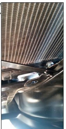
washers and insert them through the holes in the bumper with the threads facing forward. Do On the back edge of the bumper steel metal there are holes. Take the three bolts and
