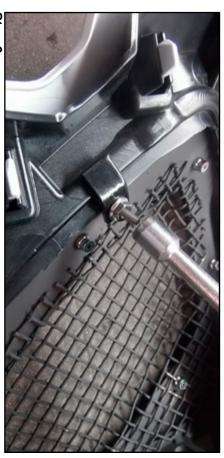
Secure grille studs with the included brackets and locknut's Step 6
