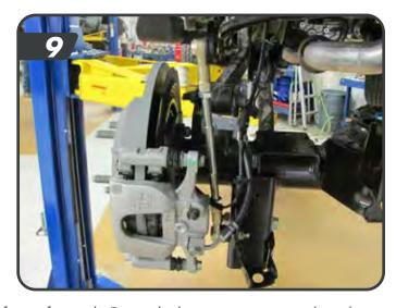
Install the rear bump stop spacers on the axle with slant cut facing forward. Fasten the bump stop spacer to the axle with the  $5/16'' \times 7/8''$  bolts, nuts and washers. Torque bolts to 15 ft-lbs. ( $\frac{1}{2}$ ") [10 - 3" extension shown]
