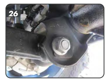
Repeat cam bolt installation on the driver's side.
