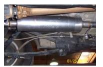
INSTALL MUFFLER #B ONTO HEADPIPE #A WITH INLET TOWARDS THE MOTOR. INLET OF MUFFLER IS LOOKING INTO THE LOUVERS USE CLAMP #E TO SECURE MUFFLER TO THE HEADPIPE. DO NOT TIGHTEN. OUTLET OF MUFFLER SHOULD BE AT THE 10 O'CLOCK POSITION.
