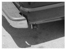
4. BEFORE INSTALLING OVERAXLE TAILPIPE. YOU MUST UNBOLT FACTORY REAR TAILPIPE HANGER AND ROTATE IT 180 **DEGREES**. Insert the overaxle tailpipe. #C no less than  $1\frac{1}{2}$ " and no more than 2". Slightly lean to the driver side. Slide turnout pipe #D on to the tailpipe. Roll turnout pipe until you have it at the correct angle for your truck. Insert welded hanger into rubber grommet. Clamp down. Using clamp #G
