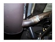
2. To remove the stock exhaust, unbolt band clamp located just behind your factory muffler.
