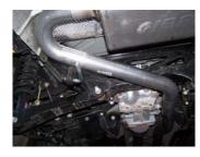
5. Slide inlet pipe #C over the intermediate pipe. Insert welded hanger into rubber grommet. Secure with clamp #G. Do not tighten.
