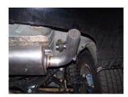
7. Slide exit pipe #E into muffler 1.5-2". Insert welded hanger into rubber grommet. Secure with clamp #G. Do not tighten.
