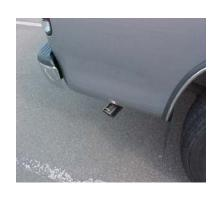
NOW INSTALL THE STAINLESS STEEL TIP USE ANY ALUMINUM OR STAINLESS STEEL CLEANER TO POLISH YOUR TIP. TIGHTEN ALL CLAMPS AND HANGERS STARTING FROM THE HEADPIPE BACK
