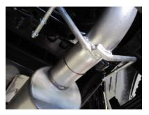
INSTALL THE OVERAXELE TAILPIPE #C INTO THE MUFFLER 1-1/2" TO 2". INSERT WELDED HANGERS INTO RUBBER GROMMET. SECURE TO THE MUFFLER USING CLAMP #E. DO NOT TIGHTEN.
