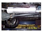
HEAD PIPE 1-1/2" TO 2" WITH THE LOUVERS FACING TOWARDS THE CONVERTER. THE MUFFLER OUTLET SHOULD BE POSITIONED AT 12:00. USE A JACK STAND TO SUPPORT THE MUFFLER. USE CLAMP #E TO SECURE THE MUFFLER TO THE HEAD PIPE. DO NOT TIGHTEN. MUFFLER INLET IS LOOKING INTO THE LOUVERS.
