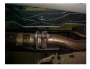
LAY OUT THE EXHAUST AND COMPARE PART NUMBERS. FOR AN EASIER REMOVAL OF THE STOCK EXHAUST CUT THE TAILPIPE BEHIND THE MUFFLER USING A HACKSAW. UNBOLT THE FACTORY FLANGE IN FRONT OF THE MUFFLER WITH OUT REMOVING THE FACTORY DOUGHNUT GASKET. YOU WILL RE-USE STOCK BOLTS. NOW REMOVE YOUR STOCK EXHAUST. LEAVE ALL RUBBER GROMMETS IN PLACE.
