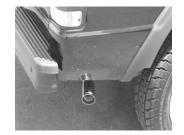
INSTALL THE STAINLESS STEEL TIP. USE ANY ALUMINUM OR STAINLESS STEEL CLEANER TO POLISH THE TIP. NOW TIGHTEN ALL CLAMPS, HANGERS, AND BOLTS.
