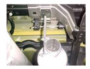
ATTACH REAR MUFFLER HANGER #H ONTO OUTLET OF MUFFLER AND INSERT WELDED ROD INTO THE RUBBER GROMMETS. THE VERTICAL ROD OF HANGER #H WILL BE POSITIONED ON THE DRIVER SIDE OF THE MUFFLER OUTLET. DO NOT TIGHTEN.
