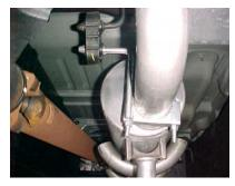
MAKE SURE YOU HAVE A 1" CLEARANCE ON ALL RUBBER BRAKE LINES, SHOCK BOOTS, TIRES, FUEL LINES, ETC..
