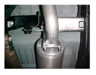
Install rear muffler hanger #F onto outlet of muffler and clamp down to tailpipe.
