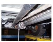
2. Bolt head pipe #A onto your existing stock front pipe and attach with factory hardware. DO NOT TIGHTEN. Use a jack stand to support the converter. Insert welded hangers into rubber grommet.
