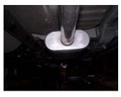
**3.** Install muffler #B onto head pipe  $1\frac{1}{2}$ "-2" with the louvers facing towards the converter. Use a jack stand to support the muffler. Use clamp #E to secure the muffler to the headpipe. DO NOT TIGHTEN.
