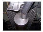
4. Install muffler #B onto headpipe  $1\frac{1}{2}$ "-2" with the louvers facing towards the converter. Use a jack stand to support the muffler. Use clamp #E to secure the muffler to the headpipe. Do not tighten. Muffler inlet is looking into the louvers. Outlet of muffler will be at approximately 2 o'clock.
