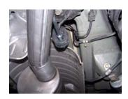
5. Install the overaxle tailpipe #C to the muffler  $1\frac{1}{2}-2^{"}$ . Use clamp #E to secure tailpipe to muffler. Insert welded hanger into rubber grommet.
