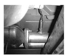
RE-INSTALL O2 SENSOR. USE A SMALL AMOUNT ANTI-SIEZE ON THE THREADS. NOW FIRMLY TIGHTEN ALL CLAMPS, HANGERS, FLANGE, AND BOLTS.
