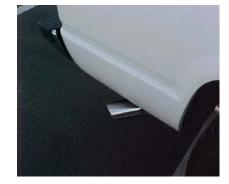
INSTALL TURNOUT PIPE #D INTO TAILPIPE USING CLAMP #G . INSTALL THE STAINLESS TIP AND CLAMP DOWN. USE ANY STAINLESS STEEL OR ALUMINUM CLEANER TO POLISH TIP. TIGHTEN ALL NUTS, BOLTS AND CLAMPS.
