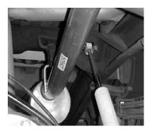
SLIDE MUFFLER WITH DUAL INLET ONTO HEADPIPE AT LEAST 1-1/2" TO 2". MUFFLER OUTLET SHOULD BE AT THE 12 O'CLOCK POSITION. USE CLAMPS #F TO ATTACH IT TO THE HEADPIPE. INSERT WELDED HANGER INTO RUBBER GROMMET. MAKE SURE INLETS AND MUFFLER IS LEVEL. USE JACK STAND TO SUPPORT MUFFLER. DO NOT TIGHTEN.
