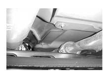
FOR EASIER REMOVAL OF THE FACTORY EXHAUST. CUT BEHIND THE MUFFLER AT THE TAILPIPE. THEN UNBOLT THE FACTORY HEADPIPE AT THE FLANGE IN FRONT OF THE MUFFLER YOU WILL BE REUSING. STOCK BOLTS.
