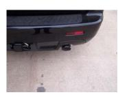
11. Install stainless steel tips. Clamp down. When you have everything in place, firmly tighten all bolts and clamps down securely. Use stainless steel cleaner and a Scotch Brite pad weekly to prevent tip from discoloration. Inspect all fasteners after 25-50 miles of operation and re-tighten as necessary.
