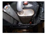
4. Install muffler onto head pipe #A. 1½"-2" with the louvers facing towards the converter. Use a jack stand to support the muffler. Use clamp #E to secure the muffler to the headpipe. DO NOT TIGHTEN. Muffler inlet is looking into the louvers. Outlet will be on the drivers side.
