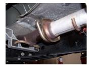
2. To remove the stock exhaust, remove it from the 2 bolt flange located in front of the muffler. Disengage the welded hangers using WD-40 from the OEM rubber grommets. Do not damage or remove the rubber grommets as you will reuse them to mount your new system. Now, cut off tailpipe before and after rear axle for removal.
