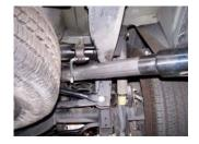
5. Install tailpipe #C into the muffler 1½-2". Insert welded hangers into rubber grommets use clamp #E to secure to muffler. Do not tighten.
