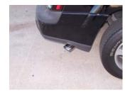
**9.** Install stainless steel tip #D. Clamp down. When you have everything in place, firmly tighten all bolts and clamps down securely. Use stainless steel cleaner and a Scotch Brite pad weekly to prevent tip from discoloration.
