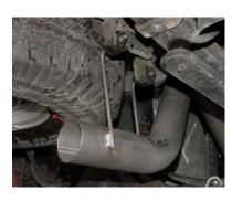
CONNECT TURNOUT #D EXIT PIPE TO THE REAR OVERAXLE PIPE. ROLL TURNOUT PIPE UNTIL YOU HAVE IT AT THE CORRECT ANGLE FOR YOUR TRUCK AND CONNECT WITH CLAMP #F. BUT DO NOT TIGHTEN.
