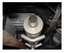
CONNECT MUFFLER#B TO THE FRONT EXTENSION PIPE WITH THE LOUVERS FACING TOWARDS THE CONVERTER. USE A JACK STAND TO SUPPORT THE MUFFLER. CONNECT WITH CLAMP #F. DO NOT TIGHTEN. MUFFLER INLET IS LOOKING INTO THE LOUVERS.
