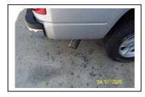
Install stainless steel tip. Clamp down. When you have everything in place, firmly tighten all bolts and clamps down securely. To clean stainless steel tip use any stainless steel cleaner.
