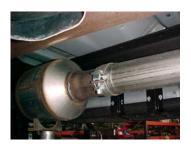
Lay out the exhaust on the floor so it looks like the drawing and compare parts with manual. To remove the stock exhaust remove it from the clamp located just behind the catalytic converter.
