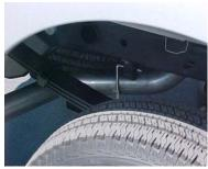
RUBBER GROMM CLAMP #E TO S PIPE TO MUFFL NOT TIGHTEN.
