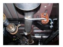
INSTALL HEADPIPE # A INTO STOCK PIPE. THE END OF THE PIPE SHOULD BE AT THE 12 O'CLOCK POSITION,. INSERT WELDED HANGERS INTO RUBBER GROMMET. ATTACH WITH FACTORY CLAMP. DO NOT TIGHTEN.
