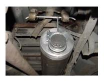
INSTALL MUFFLER #B ONTO HEADPIPE #A 1-1/2" TO 2". USE A JACKSTAND TO SUPPORT MUFFLER. SECURE MUFFLER TO HEADPIPE WITH CLAMP #I. DO NOT TIGHTEN. INSTALL HANGER #G ONTO OUTLET OF MUFFLER AND INSERT HANGERS INTO RUBBER GROMMETS. MUFFLER INLET IS LOOKING INTO THE LOUVERS.
