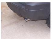
**6.** Install stainless steel tips #E. Clamp down. When you have everything in place, firmly tighten all bolts and clamps down securely. Use stainless steel cleaner and a Scotch Brite pad weekly to prevent tip from discoloration.
