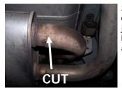
2. To remove the stock exhaust, cut off your stock over axle tailpipe just at the muffler. Then remove hangers from rubber grommets and remove muffler
