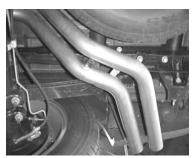
NOW INSTALL DRIVERSIDE TAILPIPE #D. THE SPARE TIRE MAY NEED TO BE LOOSENED AND PUSHED TO THE DRIVER SIDE TO ALLOW FOR CLEARANCE. USE BOLT KIT # I TO ATTACH BOTH TAILPIPES TOGETHER. DRIVERSIDE TAILPIPE BRACKET WILL BE POSITIONED ON TOP OF PASSENGER TAILPIPE BRACKET.
