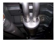
4. Install muffler #B onto headpipe #A 1.5-2" with louvers facing towards the converter. Use a jack stand to support the muffler. Use clamp #G to secure muffler to headpipe. Do not tighten.
