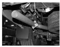
INSTALL DRIVER SIDE TAILPIPE #D INTO MUFFLER AT LEAST  $1\frac{1}{2}$ " TO 2". THIS PIPE WILL ROUTE OVER THE AXLE AND BETWEEN THE SHOCK AND SPARE TIRE. USE CLAMP #G TO SECURE PIPE TO MUFFLER. DO NOT TIGHTEN. INSERT WELDED HANGER INTO RUBBER GROMMET.
