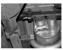
INSTALL MUFFLER #B ONTO HEADPIPE AT LEAST  $1\frac{1}{2}$ " TO 2". USE CLAMP #F TO SECURE MUFFLER TO HEADPIPE. DO NOT TIGHTEN. USE A JACK STAND TO SUPPORT THE MUFFLER. OUTLETS SHOULD BE AT THE TOP.
