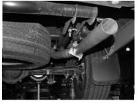
INSTALL PASSENGER SIDE TAILPIPE #C INTO MUFFLER AT LEAST 1  $\frac{1}{2}$ " TO 2". USE CLAMP #G TO SECURE PIPE TO MUFFLER. DO NOT TIGHTEN. THE TAILPIPES WILL BOTH LEAN TOWARDS THE DRIVER SIDE FOR CLEARANCE.
