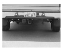
**INSTALL EXIT PIPES #E ONTO** TAILPIPES. CUT TO YOUR PREFERED LENGTH USE CLAMPS #G TO SECURE EXIT PIPES TO TAILPIPES. THESE CLAMPS ALSO ATTACH TO METAL HANGERS #H. THESE METAL HANGERS NEED TO BE ROTATED IN ORDER TO ADJUST FOR CLAMPING. NOW YOU CAN TIGHTEN ALL CLAMPS, NUTS, AND BOLTS, STARTING FROM THE FRONT WORKING BACK, USE ZIP TIES TO TIE AWAY BRAKE LINES. IF YOU WOULD LIKE YOUR EXIT PIPES TO EXIT BEHIND THE REAR WHEELS ROTATE THEM TO DO SO. INSTALL STAINLESS TIPS.
