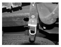
INSTALL METAL HANGERS #H INTO HOLES LOCATED APPROX. 16" FROM THE REAR OF THE FRAME. METAL HANGERS ARE MOUNTED ON THE OUTSIDE OF FRAME. USE HARDWARE KIT # I. THE BOLT AND WASHER WILL GO INTO THE 3<sup>RD</sup> HOLE FROM THE TOP OF THE HANGER.
