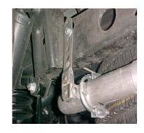
INSTALL METAL HANGER # J INTO HOLE LOCATED APPROXIMATELY 23" FROM THE REAR OF THE FRAME. USE TOP HOLE ON HANGER. INSTALL DRIVER SIDE OVERAXLE TAILPIPE # C INTO THE MUFFLER 1-1/2"-2". USE CLAMP #I TO SECURE PIPE TO MUFFLER.DO NOT TIGHTEN.
