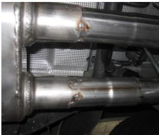
4. Install muffer #B onto headpipe #A 1.5-2". Use a jack stand to support the muffer. Use clamp #f to secure muffer to headpipe. Do not tighten.
