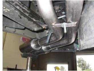
5. Install the driver side over axle tailpipe #C into muffer 1.5-2". Use clamp #G to secure tailpipe and muffer. Insert welded hangers into rubber grommets.
