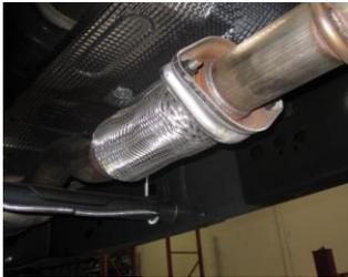
2. To remove your stock exhaust, unbolt the 2-bolt flange located in front of the muffer. For an easier removal of the factory exhaust cut off your tailpipe behind the muffer outlet. Leave all rubber grommets in place. Use WD-40 to aid in the removal of the hangers from the rubber grommets.
