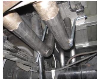
6. Install passenger side tailpipe #D into muffer 1.5-2" and attach with clamp #G. Use bolt kit #H to attach the tailpipes together. Do not tighten. Insert welded hanger into rubber grommet.
