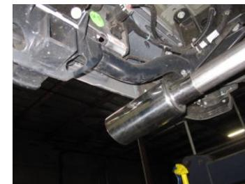
8. Install stainless steel tips. Clamp down. When you have everything in place, firmly tighten all bolts and clamps down securely. Inspect all fasteners after 25-50 miles of operation and re-tighten as necessary.
