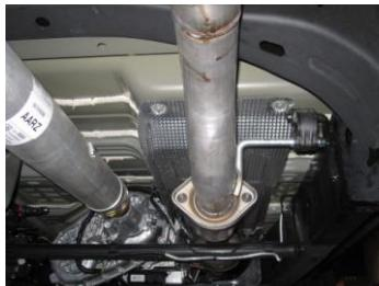
3. Install headpipe #A onto your existing stock 2-bolt flange. Use your factory nuts. Insert hanger into rubber grommet. Do not tighten.
