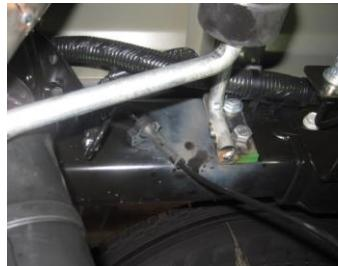
5. Install the driver side rear tailpipe hanger #F onto frame using bolt kit provided.
