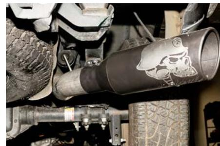
7. Be sure to check all clearance after each section has been tightened to be sure there is proper clearance. It may take 4-500 miles for your vehicle to fully adjust to the changes in exhaust flow.
