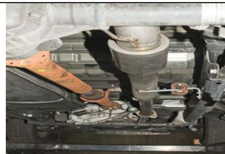
4. Install over axle pipe Item # B into the muffler outlet. Slip the hangers into the rubber grommets. Use clamp Item# D to secure and keep tailpipe loose.
