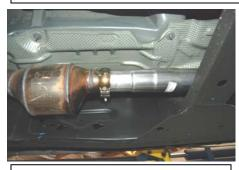
2. Install Head pipe Item # A onto the factory flange. You will re use the factory clamp at this connection. Loosely tighten down the clamp.
