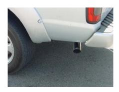
NEXT INSTALL YOUR STAINLESS STEEL TIP TO YOUR DESIRED LOOK. USE A STAINLESS OR ALUMINUM CLEANER TO POLISH TIP. NOW TIGHTEN ALL CLAMPS STARTING FROM THE FRONT AND WORKING BACK.
