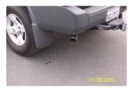
INSTALL TAILPIPE #C ONTO MUFFLER 1-1/2" TO 2". ROTATE TAILPIPE UNTIL REAR HANGER LINES UP WITH THE FACTORY GROMMET. INSTALL WELDED HANGER WITH FACTORY12MM NUT THAT YOU REMOVED FROM STEP #1. INSERT OTHER WELDED HANGERS INTO RUBBER GROMMETS. USE CLAMP #E TO SECURE TAILPIPE TO MUFFLER. DO NOT TIGHTEN.
