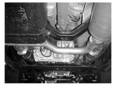
INSTALL Y-PIPE # A ONTO YOUR EXISTING STOCK FLANGES. INSERT HANGER INTO RUBBER GROMMET. USE YOUR FACTORY HARDWARE TO SECURE. DO NOT TIGHTEN.
