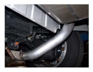
GIBSON EXHAUST systems are designed on a factory stock vehicle. Any aftermarket products installed could increase the sound levels of the exhaust. Make sure there is a 1" clearance from ALL rubber brake lines, shock boots, lines, tires, etc. to prevent heat related damage or fire.
