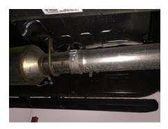
2. To remove the stock exhaust Un bolt the factory clamp located just behind the factory DPF unit. Disengage the welded hangers using WD-40 from the OEM rubber grommets. Do not damage or remove the rubber grommets as you will reuse them to mount your new system. Now, cut off tailpipe and remove exhaust. If your vehicle is on a lift or on jack stands you may not be required to cut the factory
