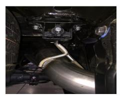
**4.** Install The Louver Exit pipe Item# B onto the Over axle pipe. Use clamp Item # D to secure the Exit pipe to the Over axle pipe. Do not tighten. Insert the Hanger into the Rubber Grommet.
