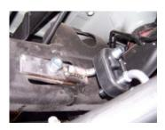
6. Install the driver side rear tailpipe hanger #H. Place the brace on the inside of the frame and the hanger portion on the outside of the frame Secure with supplied bolt kit.
