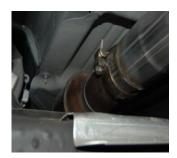
2. First remove hardware at the 2-bolt flange located in front of the muffler. Save the stock hardware as you will reuse it to attach new headpipe. Disengage the welded hangers from the OEM rubber grommets. Use WD-40 to aid in this process. Do not damage or remove the rubber grommets as you will reuse them to mount your new system. Now, cut off tailpipe and remove exhaust.
