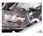
6. Install the driver side rear tailpipe hanger #H. Place the brace on the inside of the frame and the hanger portion on the outside of the frame Secure with supplied bolt kit.
