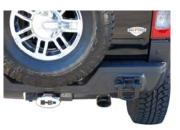
6. Install stainless steel tip. Clamp down. When you have everything in place, firmly tighten all bolts and clamps down securely. Use stainless steel or aluminum cleaner to polish tips. Inspect all fasteners after 25-50 miles of operation and re-tighten as necessary.
