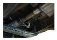
3. Slide headpipe #A onto existing stock front pipe and secure with clamp #F. Do not tighten.
